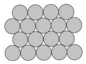
**Fig. 2.1** The densest packing in dimension two: the hexagonal lattice packing
